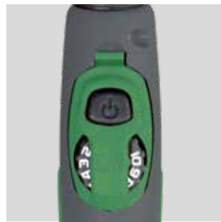
Keypad unit with horizontal TIG control knob (RH) Art. no. ....80300130 (old model) Art. no. ....80300070 (new model)
